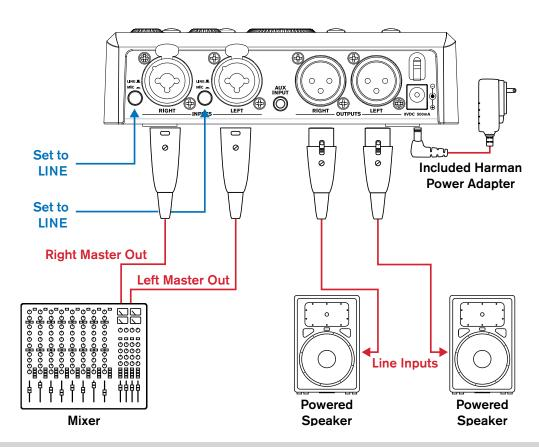
**NOTE:** For best noise performance, balanced cables (XLR or 1/4" TRS Phone) should be used between the mixer and goRack if the mixer's outputs are balanced. See **'Audio Cable Diagrams' on page 26** for more information on these cable types.
