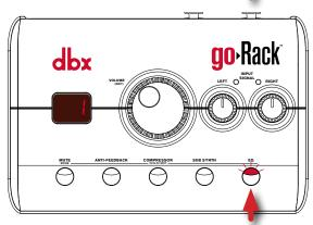
3. While auditioning the sound system, turn the VOLUME (EDIT) encoder and select the EQ curve that sounds best for the application.
