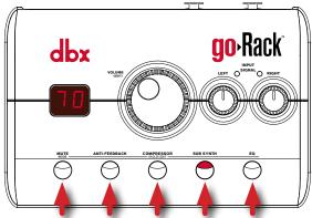
**IMPORTANT!** The subharmonic synthesis process produces low-frequency audio signals that some speakers may not be designed to reproduce. Attempting to achieve enhanced low end with these systems may not be possible and may result in over-stressing your loudspeakers. If you can't hear a discernable difference when raising the sub synth effect, it is recommended that you disable the effect. For best results, subwoofers should be used with the sub synth effect.
