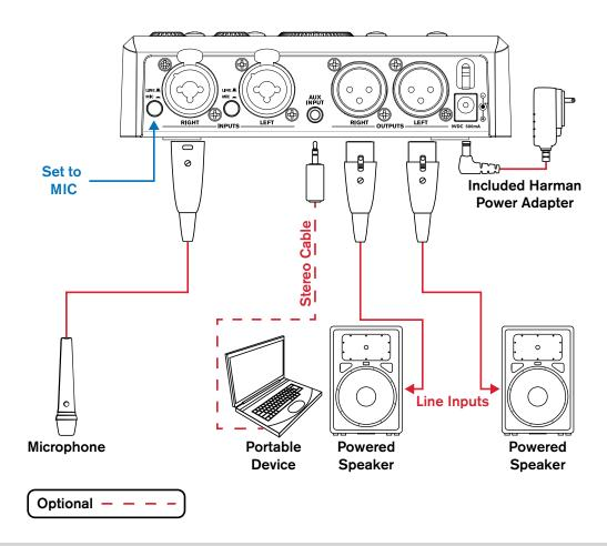
**NOTE:** A stereo (Tip-Ring-Sleeve) Mini cable should be used for the connection between the portable device and AUX INPUT. See 'Audio Cable Diagrams' on page 26 for more information on these cable types.
