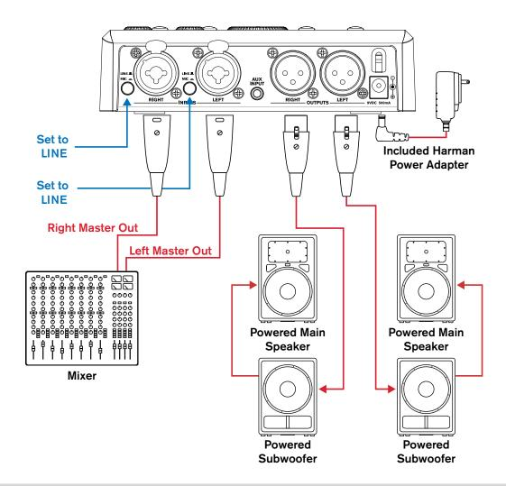
**NOTE:** For best noise performance, balanced cables (XLR or 1/4" TRS Phone) should be used between the mixer and goRack if the mixer's outputs are balanced. See 'Audio Cable Diagrams' on page 26 for more information on these cable types.
