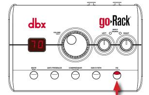
2. To change the EQ setting, press and hold the EQ button for 2 seconds (the EQ LED will flash, indicating EQ Edit mode is active).
