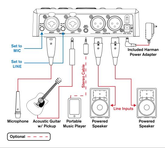
**NOTE:** A stereo (Tip-Ring-Sleeve) Mini cable should be used for the connection between the portable music player and AUX INPUT. If connecting instruments to the goRack's LEFT/RIGHT inputs using 1/4" plugs, unbalanced TS (Tip-Sleeve) instrument cables should be used. See 'Audio Cable Diagrams' on page 26 for more information on these cable types.
